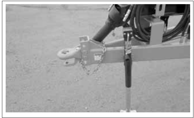
FIG. 9 FRAME LEVELING CLEVIS
