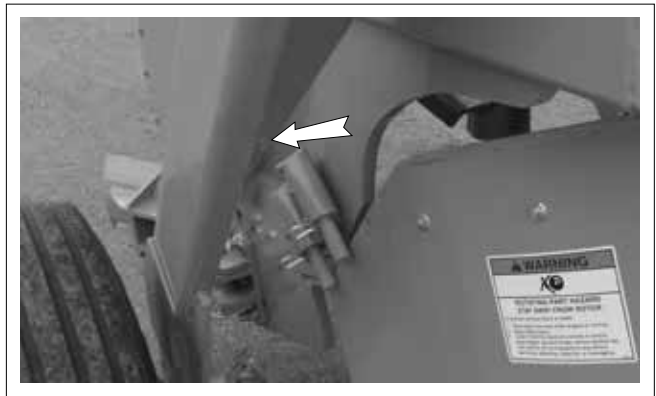
FIG. 49 CHAIN CASE LEVEL PLUG
